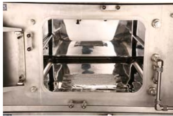
Adhesive sample inside of a small environmental chamber. © 2011 Air Quality Sciences, Inc.
