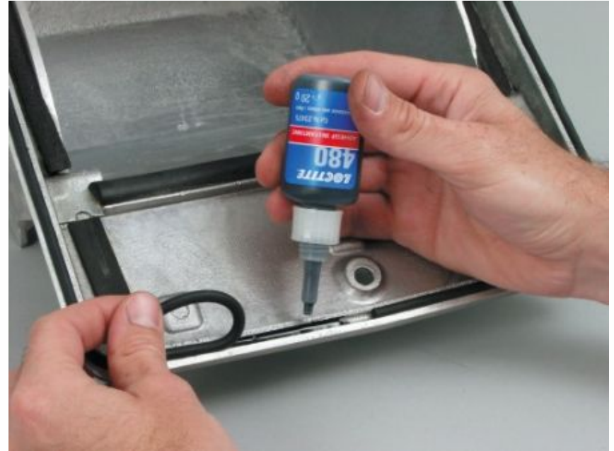
Tacking O-ring in Groove
